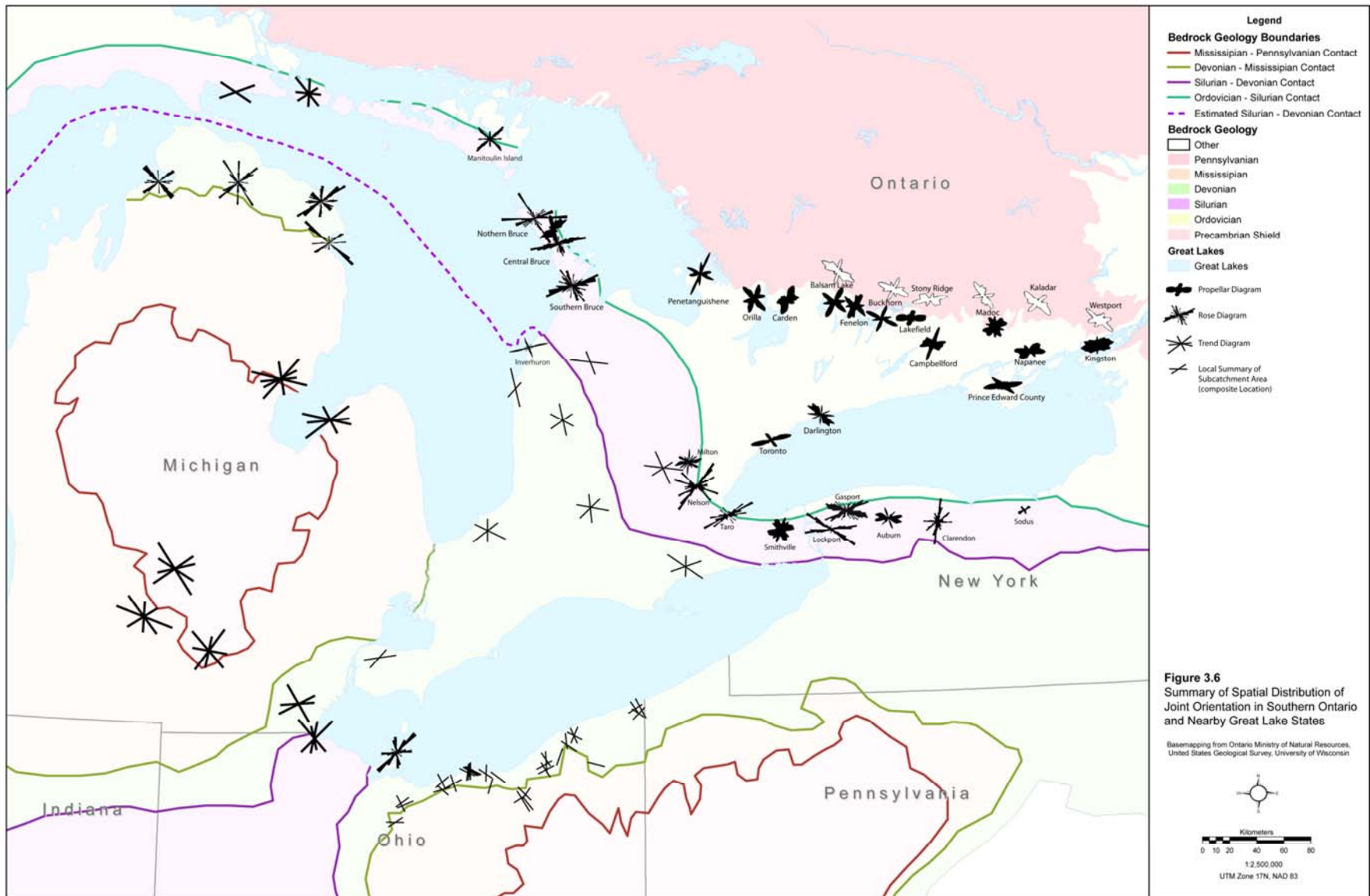
Figure 3.6 Joint Orientations of Southcentral Ontario plotted as Gaussian contoured and smoothed rose diagrams for the Paleozoic cover and Precambrian basement (Regional Geomechanics, GLL, 2008).
